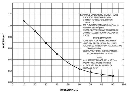
FIG. 2 Standard Radiant Heat Energy Flux Profile
