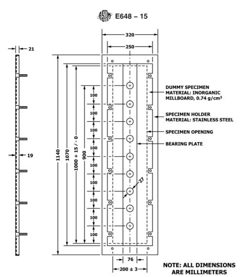
FIG. 5 Dummy Specimen in Specimen Holder (Bottom View)
