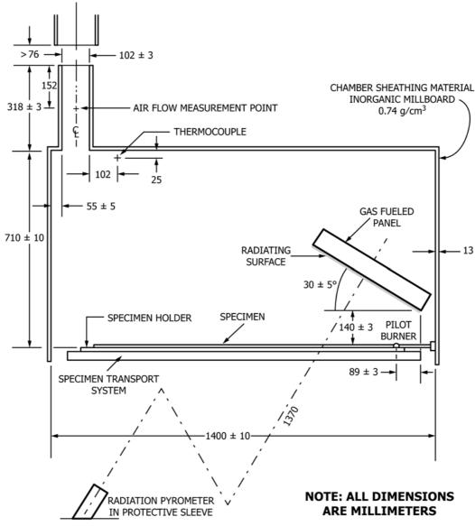
FIG. 3 Flooring Radiant Panel Tester Schematic Side Elevation
