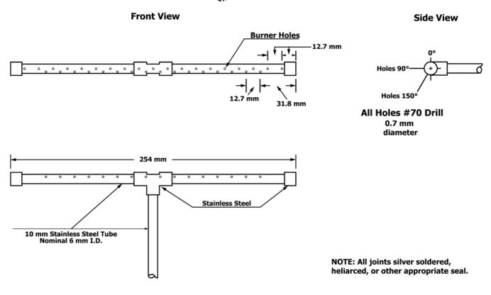
FIG. 6 Pilot Burner
